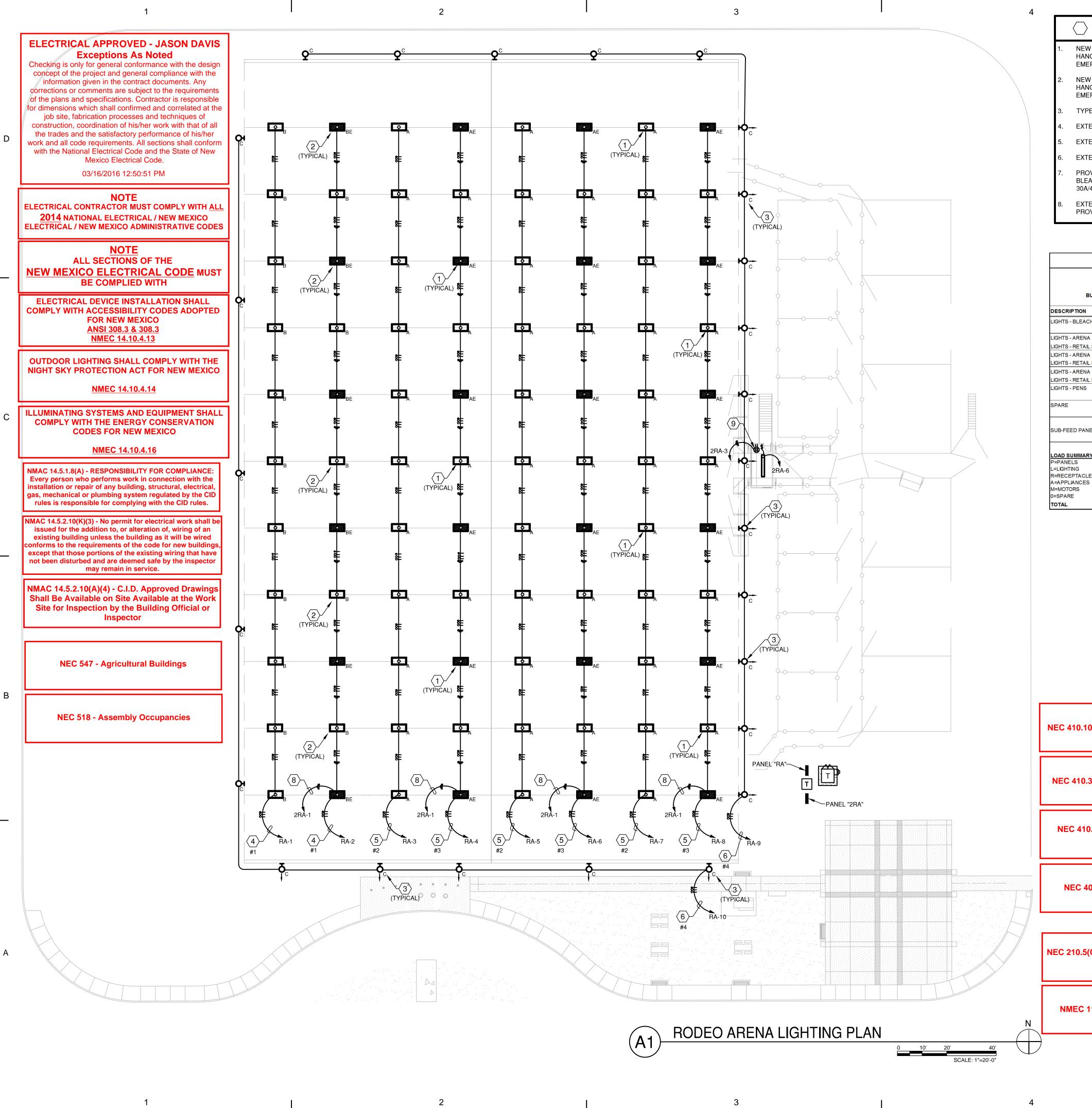
NEW TYPE "A" FIXTURE SHALL BE LITHONIA #IBL-48L-ND-SD125-HVOLT-LP840-LAH02ZU WITH TWO (2) #THUN TONG HANGER BRACKET AND #MS1360IMP, SIMILAR AND EQUAL. TYPE "AE" FIXTURE SHALL BE PROVIDED WITH #I2412 EMERGENCY LED BATTERY PACK.
